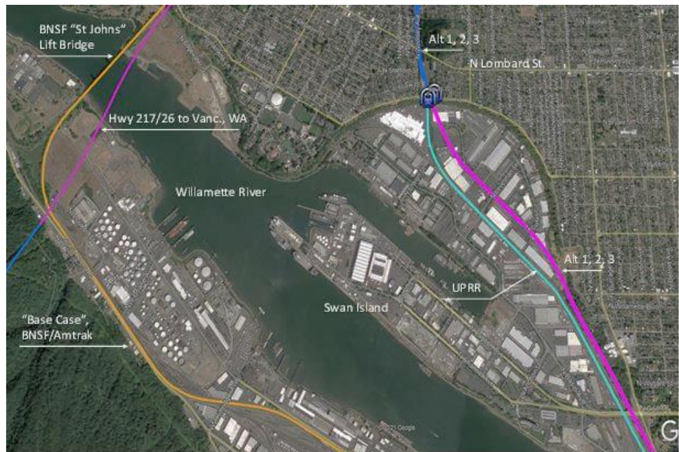
Exhibit 3-6: CHSR vs. Existing BNSF/Amtrak Alignment showing St. Johns Bridge crossing on the Existing Route
